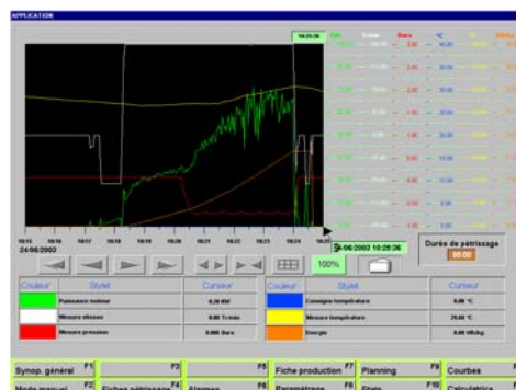
Example of measures performed in real time under vacuum on a horizontal kneader VeryMix III
